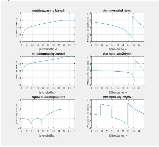
**Result:** Hence an IIR high pass digital filter is designed and its frequency response is observed using MATLAB.
