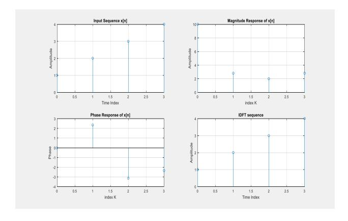
**Result:** Hence DFT and IDFT of given sequence is performed and outputs are observed using MATLAB.
