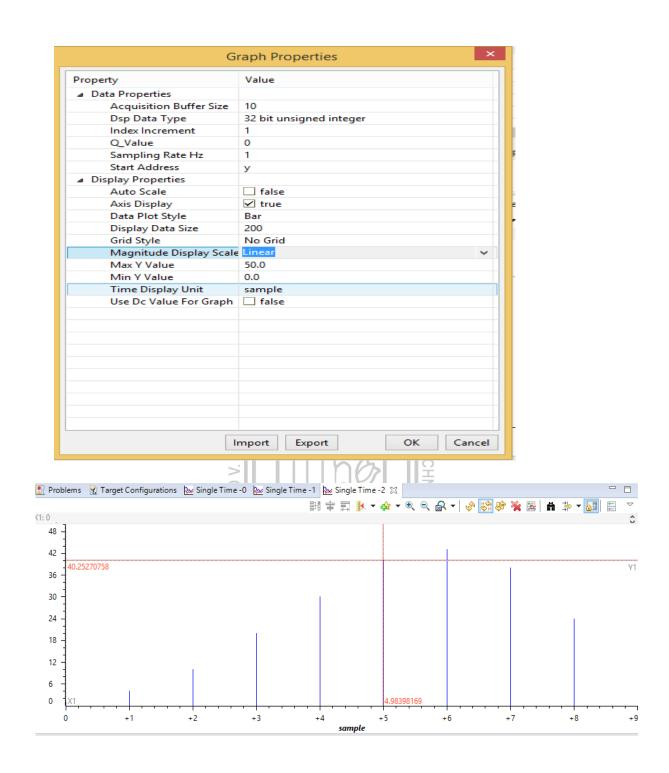
**Result:** Hence linear convolution of given sequences is performed and output is observed using TMS320C6713 DSP starter kit.
