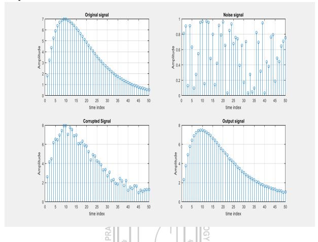
**Result:** Hence M-point Moving average filter is designed and output is observed using MATLAB.
