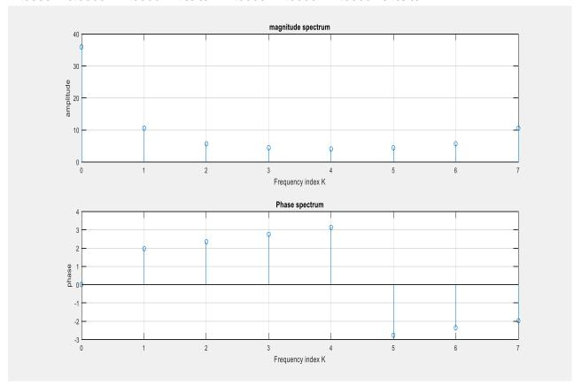
**Result:** Hence Fast Fourier transform of a given signal is computed and its spectrum is plotted using MATLAB
